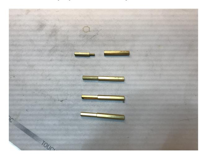
**Step 9 - Screw the 18mm & 30mm standoffs together**Connect the M2.5, 18mm Male to Female Standoffs to the M2.5, 30mm Female to Female standoffs.
