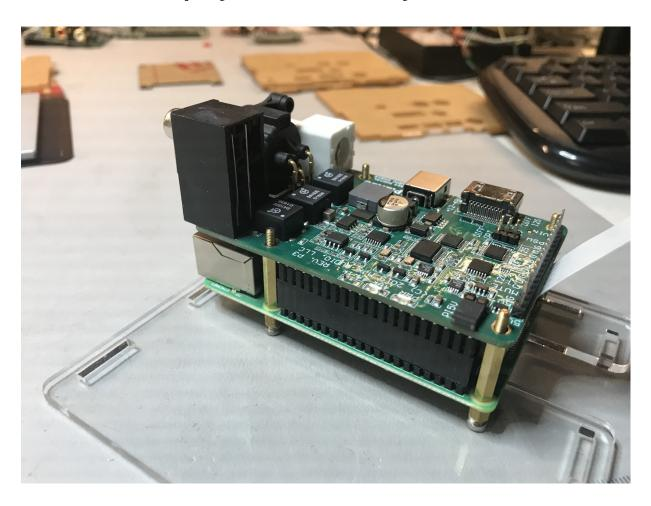
Step 5 - Attach the PI2AES to the Pi (3 or 4)
