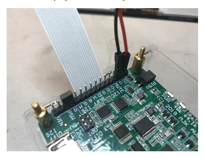
**Step 7 - Connect LCD Power to PI2AES**
